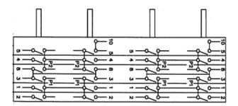
Mounting dimensions: 60mm between shaft centres. M12 centre nut mount
