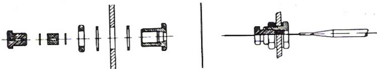
Alternatively where the vat has a 3/8 BSP socket, Fit gland adaptor EF1234.1
