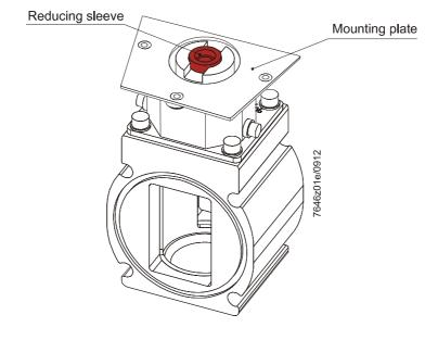
Commission the proportional controlling element only when mounting plate, flange and the respective actuator are correctly assembled.
